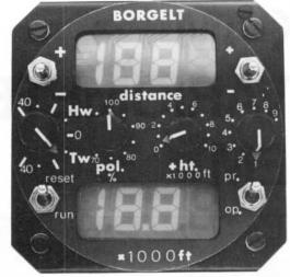
NAV, DISTANCE TO GO, ALTITUDE REQUIRED, % POLAR, HEADWIND - TAILWIND, HEIGHT, WAYPOINT SELECTOR (9 DISTANCES)
