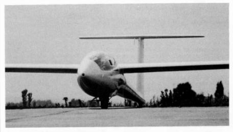
With triangular flap retracted, above, and extended, below, 21% change in wing area is readily apparent.
