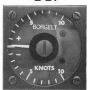
VARIOMETER, 1 - 2 SECOND RESPONSE TIME, SELECTABLE DURING FLIGHT, THREE STAGE GUST FILTER.
